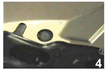
Remove six pushpins from the bottom side of the fascia. Set the pushpins aside to be reinstalled later.
