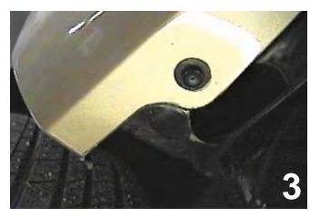
3. Using the 10MM socket, remove the metric bolt from the bottom side of the fascia corner. Set the metric bolt aside to be reinstalled later. Do this to both sides of the vehicle.
