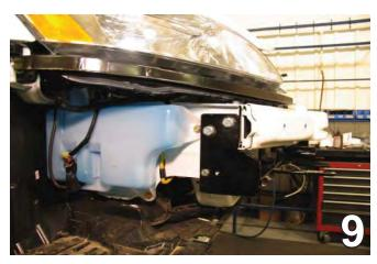
Reinstall the fascia and headlight assemblies.Some trimming may be required.
