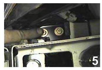
5. Using the 10MM socket, remove five bolts under and one on the outside of the headlight assemblies, unplug and set aside to be reinstalled later. Set metric bolts aside to be reinstalled later. Do this to both sides of the vehicle.
