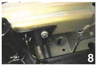
8. Reinstall the metal bumper, align the 3/8-16 nutplate inside the metal bumper with the drilled 13/32" hole and tighten the 1/2" lock washer, 3/8" lock washer. for upper supports.
