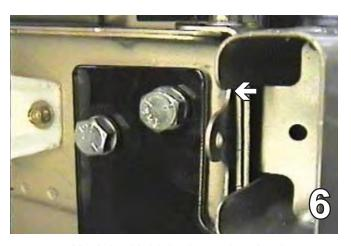
6. **2002 Models:** Hold the baseplate in place, clamp with the vise grips, and center to the bottom of the metal bumper.
