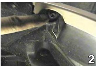
Using the 8MM socket, just behind the fascia's upper corner, remove one metric bolt. Set the bolt aside to be reinstalled later. Do this to both sides of the vehicle.
