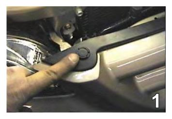
Remove two pushpins from the top side of the grille. Set the pushpins aside to be reinstalled later.
