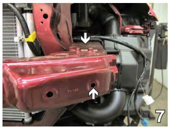
Using a 12Mm socket remove two metric bolts from the top of the metal bumper and on the bottom.
