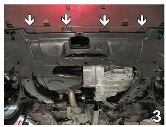
3. Remove four push pins from the lower edge of fascia and belly pan.
