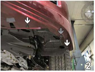
Using 10MM socket remove two metric bolts from the lower edge of the fascia just forward of the front tire, as indicated by the white arrows in the photo above. Remove one push pin indicated by the grey arrow in the photo above. Do this to both sides of the vehicle, the driver's side is shown.
