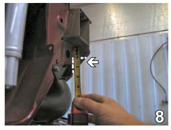
Measure 1 1/4" down from the bottom of the frame rail. Make a horizontal mark on the webbing back to cross member and down. Using a reciprocating saw remove this portion of the frame. Do this on both sides, the driver's side is shown.
