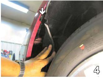
4. Just forward of the front tire on fascia's corner, remove on Phillips head screw with the Phillips screw driver. Do this to both sides of the vehicle, the driver's side is shown. Pull the fascia corner out to the side of the vehicle and then forward to release, set fascia aside carefully.
