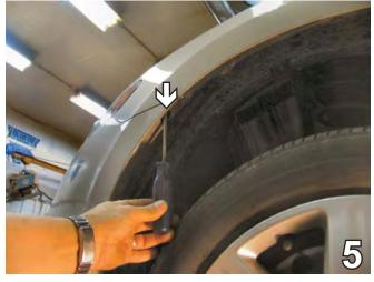
Just forward of the front tire, in an opening between the front fascia and the wheel well, use a Phillips screwdriver to remove the screw. Do this to both sides of the vehicle. Set screws aside to be reinstalled later.
