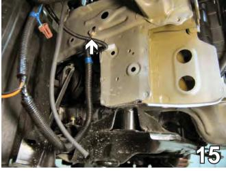
Relocate and secure the ground wire to the upper rear section of the frame rail on the passenger's side.
