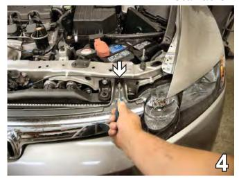
4. Above the grille, next to the radiator support bracket, use a T30 Torx Socket to remove the metric bolt. Do this to both sides of the vehicle. Set screws aside to be reinstalled later.
