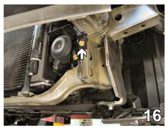
16. Using the 12MM socket, remove the metric bolt from the horn shield on the radiator support on the passenger's side. Hang horn over the lower radiator support ensuring it is out of the way.
