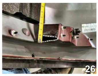
26. On the backside of the fascia, using a utility knife, cut an opening to allow for the fog lights when reinstalling the front fascia. Make a vertical cut of one inch. Make two horizontal cuts (shown) of approximately two inches. Do this to both ends of the fascia.
