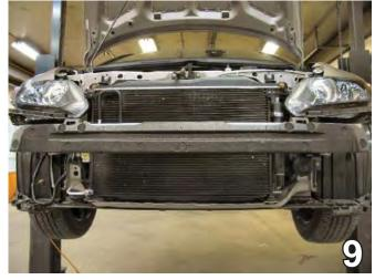
9. To remove the Styrofoam bumper, pull it forward to release it from the metal bumper.
