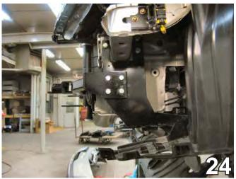
24. Slide the baseplate endplate to the outside of the support plate and align with the existing four holes of the support plate. Ensure baseplate is level with the vehicle and tighten all bolts.
