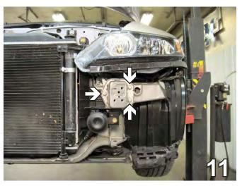
11. Using a 12MM socket, remove three metric bolts from the bumper bracket to gain access to the frame rail. Do this to both sides of the vehicle. Set bolts and brackets aside to be reinstalled later.
