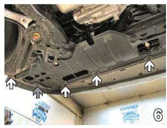
6. Along the bottom edge of the fascia, remove eight push pins, as indicated by the white arrows in the photo above. Do not remove the pushpin found second from either outer edge of the fascia as indicated by the grey arrow in the photo above.
