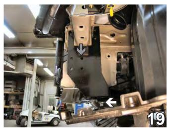
19. On the driver's side, place the support plate against the radiator support and frame. Guide upward until it surrounds the frame side extension. Hold the endplate steady and insert the existing metric bolt, from step 19, underneath the endplate and up into the bolt hole for the lower suspension, as indicated by the white arrow in the photo above. Tighten with the 17MM socket. Do not over tighten as the endplate may need minor adjustments.
