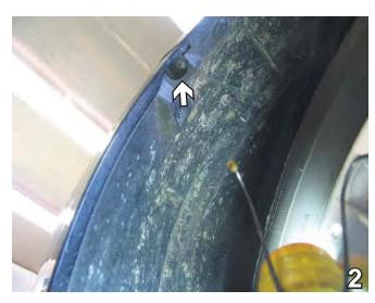
Just inside wheel well, on edge of fascia, remove one Phillips screw. Do this to both sides of the vehicle. Set screws aside to be reinstalled later.
