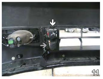
11. On the driver's side, mark the upper air vent flush with the back side of the grille opening. Using the utility knife, trim the marked area. Some models may need to have the lower air vent removed also (see gray arrow).
