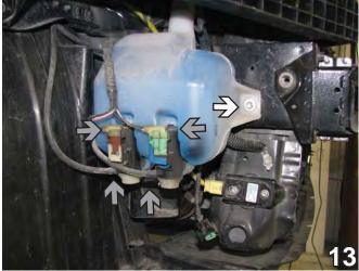
13. On the passenger side, unhook and plug the hoses and disconnect the electrical wires (gray arrows). Remove one bolt from the side of the metal bumper using the 10mm socket (white arrow). Set bolt aside to be reinstalled later.
