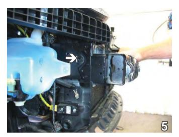
5. On the passenger side, remove one bolt from the side of the metal bumper using the 12mm socket. Set bolt aside to be reinstalled later.
