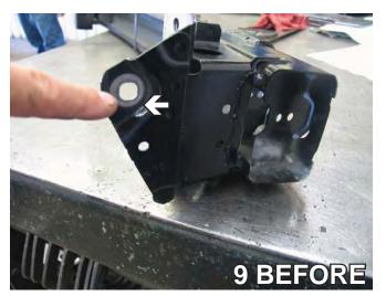
9. Flatten bumper bracket with a hammer.
