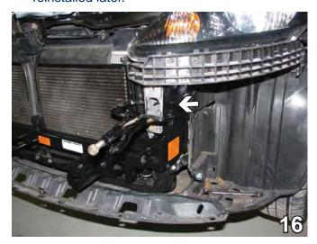
16. On the driver's side, use the baseplate as a template to drill the front bottom hole in the frame with the 13/32" drill bit. Insert 3/8-16 nut plate through frame end hole and align to the drilled hole. Install 3/8-16 x 1 ½" hex bolt with 3/8" lock washer and tighten with loctite to the nut plate.
