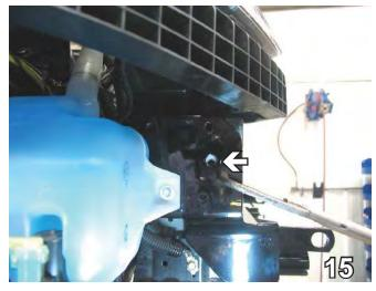
15. Align the baseplate with passenger side existing hole, flush with the top and front edge of the frame rail. Clamp in place using the vice grips. Install the 6mm hex bolt with 6mm lock washer and 1/4" flat washer to the existing hole and tighten with loctite. Using the baseplate as a template, drill the three remaining holes in the passenger's side frame with the 13/32" drill bit.
