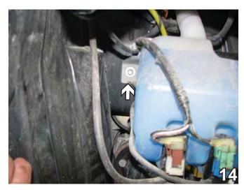
14. Using the 10mm socket, remove one bolt from the back of the washer reservoir. Set the bolt and the washer reservoir aside to be reinstalled later.
