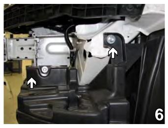
6. On the driver's side, use a 10MM socket to remove the two bolts holding the air baffle. Don't remove the air baffle just pull it back out of the way. Set the bolts aside to be reinstalled later.
