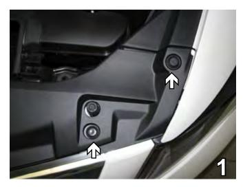
Remove two push pins from the side in order to remove the radiator cover. Do this to both sides of the vehicle. Set push pins aside to be reinstalled later.
