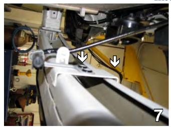
Behind the bumper, disconnect the temperature sensor by removing two push pins before taking the bumper off.
