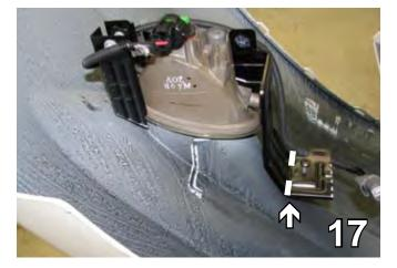
17. On the passenger side, trim the fog light bracket along the bend.
