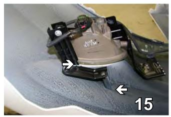
15. On the fog light bracket on the back side of the fascia, cut across the top of the lower bracket and the plastic tab and remove on the driver's side only.
