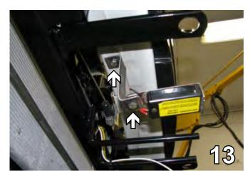
13. Reinstall the bumper. Center the breakaway bracket between the tab and the rod. Using a 13/32" drill bit, drill a hole in the bottom of the bumper. Attach the bracket with a 1/4-20 x 3/4" bolt and 1/4-20 nut. Attach the breakaway also with a 1/4-20 x 3/4" bolt and 1/4-20 nut.
