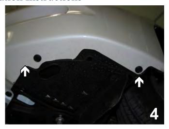
4. Underneath the fascia, remove ten push pins all the way around. Set push pins aside to be reinstalled later.
