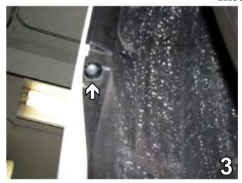
In the corner of the fascia, remove the Phillips screw. Do this to both sides of the vehicle. Set screw aside to be reinstalled later.
