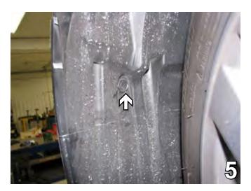
On the driver's side, remove the push pin just forward of the front tire in the wheel well. Set the push pin aside to be reinstalled later.
