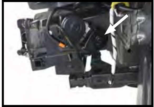
18. Reinstall the air horn to the original location. It may require bending slightly to allow for ample clearance.
