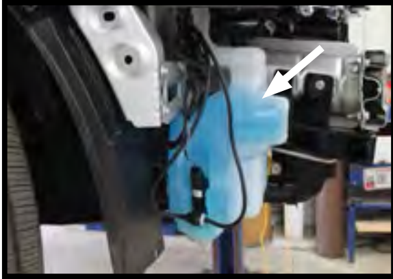
17. Reattach all electrical wiring and fluid lines.
