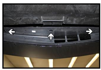
3. Remove the three (3) push pins from the underside of the fascia.
