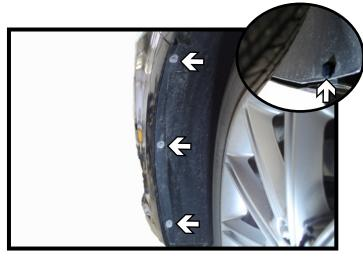
Using a 5.5MM socket, remove the three
