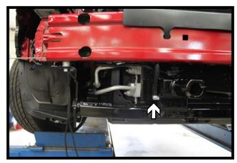
13. Using a 17/32" drill bit, drill a hole thru the bumper using the tube as a guide. Install a 1/2" x 5" bolt with flat and lock washer into the hole and a 1/2" nut plate in the bumper. Depending on the fit, 1/2" flat washers may need to be used in between the bumper and tube. Do this on both sides of the vehicle.
