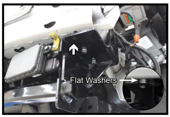
12. Using a 13/32" drill bit, drill the bottom front hole on both sides of the vehicle. Install 3/8" x 2" bolts with lock washers into the holes using flat washers in between the baseplate and frame as spacers (approximately six per side) and 3/8" nut plates in the bumper.
