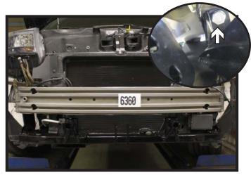
12. Install the baseplate onto the frame and clamp in place. Install the 3/4" bolt and lock washer into the existing hole on the under side of the frame (inset). Insert the 3/4" nut plate on the inside of the frame, level the baseplate and loosely tighten the bolt. Do this on both sides of the vehicle.
