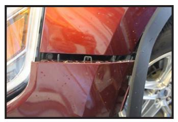
5. Lift up on the corners of the fascia to unsnap and pull it away from the vehicle disconnecting any electrical connections and fluid lines. Set the fascia aside.
