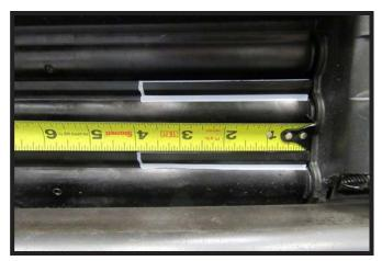
Using a reciprocating saw, trim the bottom two shutters, 4" across and roughly 1/2" deep. Do this for both sides of the vehicle.
