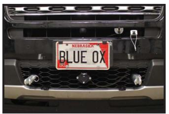
Hold the fascia as close to its original position, mark and trim the fascia around the convenience links and attachment tabs. Reinstall the fascia. Note: The fascia will fit snuggly when reinstalled.
