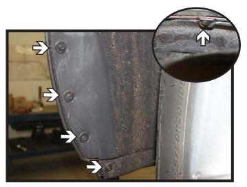
Using a 5.5MM socket, remove the seven (7) screws from the edge of the wheel well. Then above the center of the wheel, remove the push pin (inset). Do this on both sides of the vehicle.
