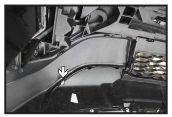
17. On the backside of the fascia trim the outer tab shown flush with the backside of the fascia for clearance of the baseplate. Do this on both sides of the vehicle.
