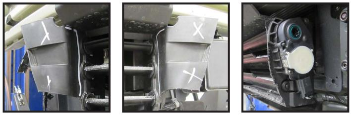
11. Using a reciprocating saw, trim the marked areas beside the shutters. On the driver side, ensure the cutting is performed against the contour of the motor.
