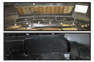
8. Using a reciprocating saw, trim the marked areas on the fascia, ensuring to not cut completely through the fascia.
