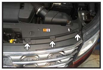
Using a 10MM socket, remove the seven (7) screws from the top edge of the fascia. There are three (3) on the driver side and four (4) on the passenger side.
