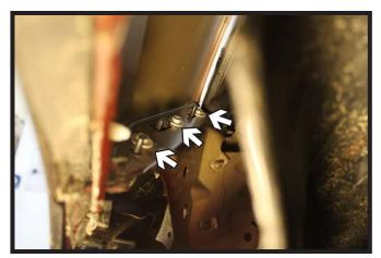
3. Using a 10MM socket, pull back the wheel well liner and remove the three (3) screws from the fascia joint. Do this on both sides of the vehicle.
