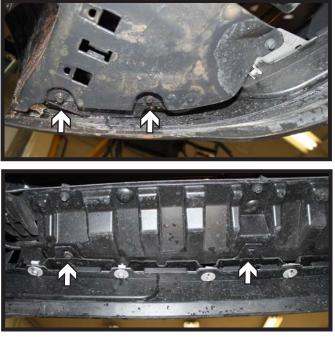
Using a 8MM socket, remove the seven (7) screws from the underside of the fascia. There are two (2) in each corner and three (3) across the front.
