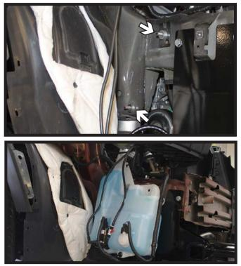
Install nine (9) 1/4" washers onto the two (2) studs for the washers reservoir (top). Reinstall the washer reservoir onto the studs and reinstall the factory nuts. The factory screw will not be reinstalled.
