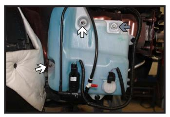
Using a 11MM socket, remove the two (2) nuts from the washer reservoir (white). Then using a 8MM socket, remove the screw (gray). Disconnect/plug all lines and set the reservoir aside.
