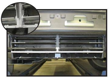
Using a reciprocating saw, trim the marked area to be flush with the shielding. Also, trim the middle plastic about 1-1/2" up to the bottom shutter, ensuring it is also flush with the plastic shielding.
