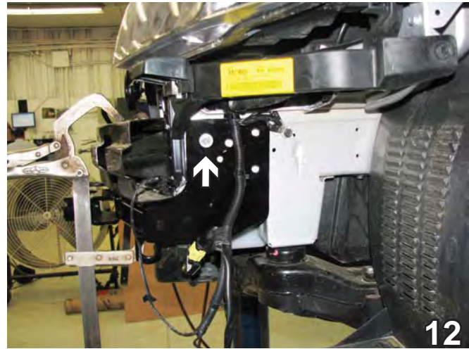
12. Slide the base plate up and align with the existing holes. Insert a 6MM-1 x 30MM bolt into the existing hole on the driver's side. On the passenger side, use a 6MM-1 x 45MM bolt. Tighten. Be sure the base plate is level with respect to the vehicle frame. Do this on both sides of the vehicle.
