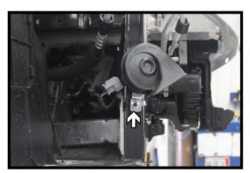
Using a 10MM socket, remove the nut from the horn bracket on the passenger side and move the horn aside.
