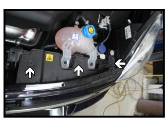
1. Using a T27 Torx, remove the six (6) screws from the top edge of the fascia. There are three (3) on each side.
