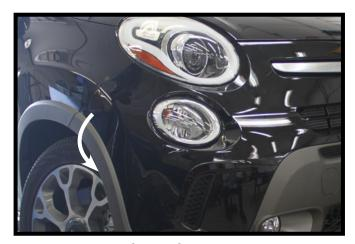
4. Unsnap the fascia from each side. Unplug all electrical connections, then pull the fascia forwards from the vehicle.
