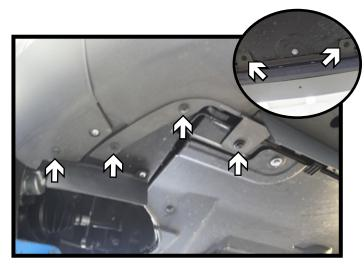
3. Using a Philips screwdriver, remove the ten (10) screws from the underside of the fascia. There are four (4) on each corner and two (2) in the middle.
