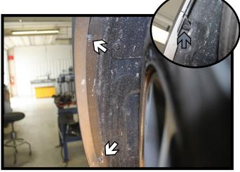
2. In the wheel well, using a Phillips screwdriver, remove the two (2) screws from the outer edge (white). Then using a T27 Torx, remove the screw from the top outer edge (gray).
