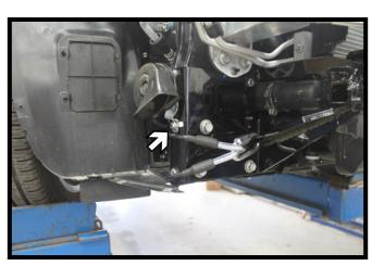
9. On the passenger side, reinstall the horn to the existing stud.
