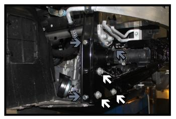
8. Slide the baseplate onto the vehicle.
