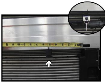
11. Optional: If installing a breakaway, measure over 5-1/4" from the slot on the driver side of the bumper. Screw the bracket to the bumper with the #10-16 self tapping screw. Install the breakaway to the bracket with a 1/4"-20 bolt and lock nut.
