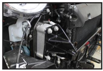
8. Install the baseplate onto the vehicle, using the existing spacer and 10MM bolts. Repeat on the other side of the vehicle. Tighten down baseplate to the vehicle.
