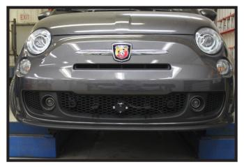
10. Hold the fascia up to the vehicle as close to it's original position. Mark and trim with a utility knife until the fascia is clear of the attachment tabs and convienence links. Reinstall the fascia.
