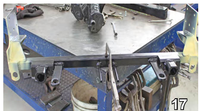
17. Lay baseplate in upright position on a smooth work surface (yellow is used on this baseplate for demonstrative purposes only). Anchor baseplate to work surface with vice grips.
