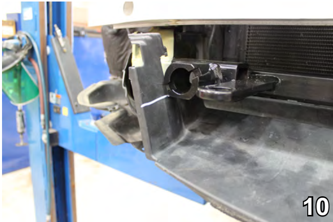
10. Detach and remove bellypan from underneath the metal bumper. Set aside to be reinstalled later.
