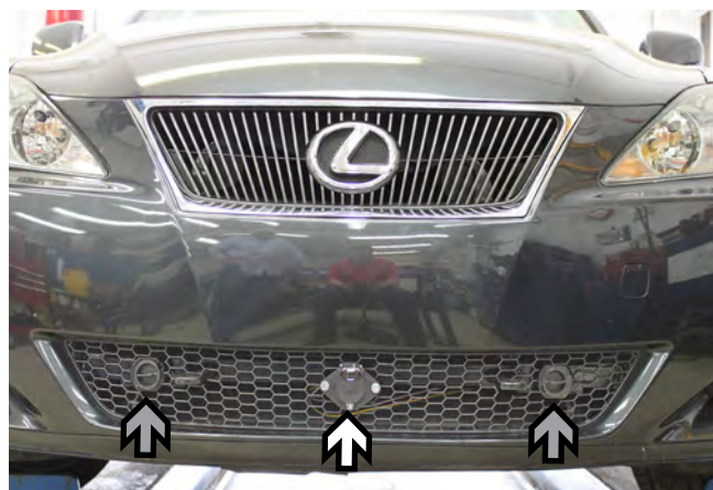
30. Reinstall foglights and connect sensor back onto fascia. Align the fascia to its original position and trim the opening for the attachment tabs with diagonal cutters (gray arrows). Do this on both sides of the vehicle. Optional: Attach the electrical bracket to the center of the fascia (white arrow). - Photo at left.
