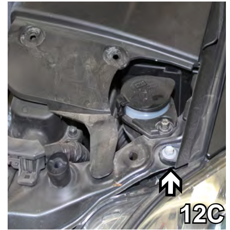
12. To remove washer fluid reservoir, with a 10MM socket, remove bolt in back (12A), in front and to the left of the reservoir (12B) as well as on the topside of the reservoir just above headlight (12C). Disconnect electrical, and plug fluid lines and set aside to be reinstalled later. NOTE: Two of the Three existing bolts will be replaced with bolts provided (12A and 12B).
