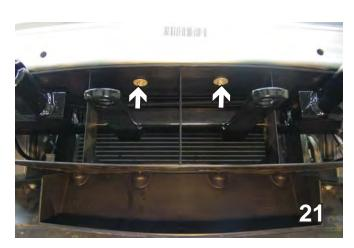
21. Reinstall bumper and air baffle over the top of the base plate. Attach with two center bolts.
