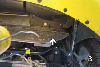
Using a flat screwdriver, remove 3 push pins from up underneath. Set push pins aside to be reinstalled later. Do this to both sides of the vehicle.
