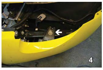
4. There is a bolt just below headlight assembly and behind fascia to be removed with a 10MM socket. Remove bolt and set aside for later reinstallation. Unhook the marker lights.
