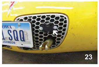
23. Cut a hole in the grille for the electrical plug to go through. Place electrical connector bracket on the back side of the grille and attach with 1/4"-20 x 1 1/2" hex bolts, flat and lock washers and 1/4"-20 whiz nuts.
