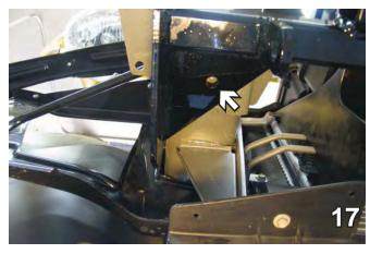
17. On the passenger side, use a 13/32" drill bit to drill a hole.
