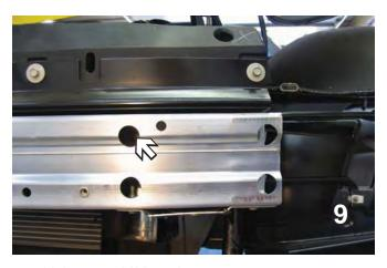
Using a 13MM socket, remove two more bolts from both sides. Set bolts aside to be reinstalled later.
