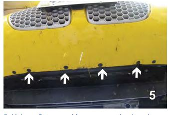
5. Using a flat screwdriver, remove the 4 push pins from the center of the fascia. Pull fascia corners out to the side of vehicle, then pull fascia forward and carefully set aside fascia and push pins for later reinstallation.
