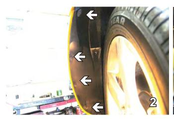
2. Using a 7MM socket, remove the 4 hex bolts just forward the front tire. Do this to both sides and set aside for later reinstallation.
