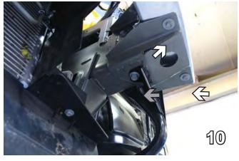
10. Remove three bolts underneath the bumper. Use a 10MM socket on the top two and a 15MM socket for the bottom one (grey arrow). Set aside bolts for later reinstallation.
