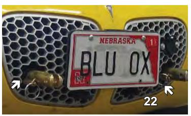
22. Hold fascia as close to its original position as possible and cut a hole in the grille with a hack saw blade for attachment tab receivers to come through. Do this to both sides. Then reinstall fascia.
