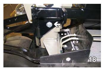
18. Insert 3/8" nut plate into frame end to align with drilled hole and tighten 3/8"-16 x 1 1/2" hex bolt, 3/8" flat and lock washer with Loctite Red.
