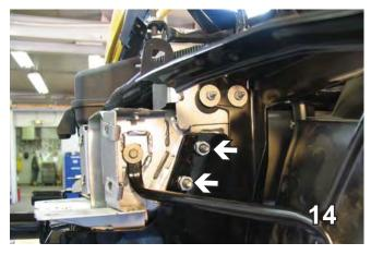
14. On the driver's side tip base plate so that hole starts on these two studs. Hand tighten the two 10M hex nuts and lock washers.
