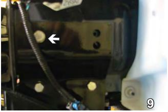
9. Slide baseplate onto the frame rail and up to bottom of metal bumper, clamp baseplate to bumper with vise grip, both sides. Align baseplate to existing bolt location for the horn bracket on the driver's side, replace and tighten existing metric bolt for horn bracket to hold baseplate in place. Be sure to align lower holes of baseplate to the center of lower frame webbing before drilling holes. Align
