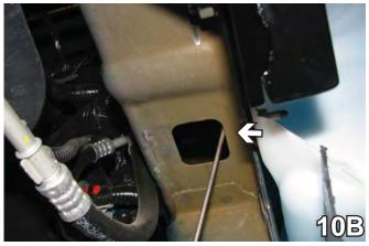
10. Using the baseplate as a template, drill a hole into the bottom of metal bumper with the 13/32" drill bit, both sides. Insert the 3/8" nut plate with the 12" wire into the open end of metal bumper to align with drilled hole, tighten 3/8-16 x 1 1/2" hex bolt and 3/8" lock washer with the 9/16" socket, both sides. Be sure and use loctite red on all bolts before tightening. Tighten all bolts according to torque chart in the General Instruction sheet.
