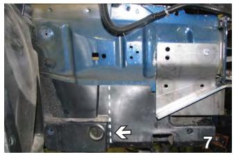
On the passenger side, using a utility knife, cut the plastic straight up next to the extended tab, as shown, and remove for nut plate insertion.
