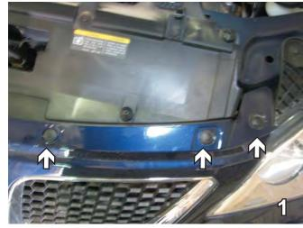
Remove the six push pins, three on each side, from the top edge of fascia just between headlight assemblies. Set pins aside to be reinstalled later.
