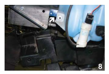
8. On the driver's side, using a utility knife, cut the plastic straight down even with the edge of the washer reservoir and remove.
