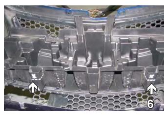
6. On the back side of the fascia, using the utility knife, cut the two outside tabs down 1 1/4".
