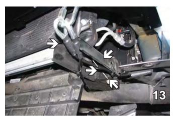
13. Attach permanent baseplate safety cables to the convenience link on the baseplate. Wrap the cables around the vehicle frame. Additional options may interfere with suggested mounting, in this case secure the cables to a solid piece of the frame as described in instructions included with the permanent baseplate safety cables. Be sure the safety cables do not rub against any hoses or moving parts. Do this to both sides of the vehicle.
