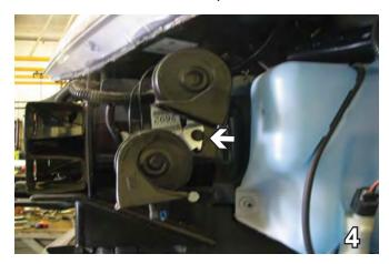
4. Using the 10MM socket, remove metric bolt from horn bracket on the driver's side and set assembly aside to be reinstalled later.
