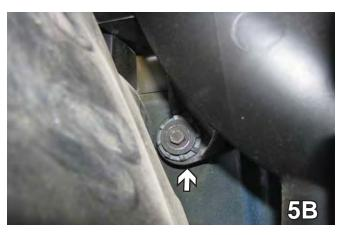
On the passenger side, remove the push pin from the front of the air baffle. Using a 10MM socket, remove one metric bolt from the back. Set assembly aside to be reinstalled later.
