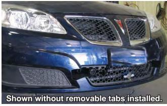
If the baseplate is in an accident, it must be replaced. DO NOT use it again! An accident can cause unseen damage and using it again could result in more damage or serious injury. DO NOT use the paseplate if it is damaged or missing parts
