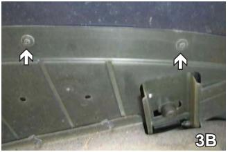
3. On the lower edge of the fascia, just forward of the front tire, using a 7MM socket remove one metric bolt (white arrow). Continuing around, remove two push pins (gray arrows). Using the 7MM socket, remove five metric bolts (3B). Remove two more push pins and one more metric bolt. Pull the corners of the fascia to the side of the vehicle to release the tabs. Pull fascia forward and carefully set fascia and bolts and pins aside to be reinstalled later.
