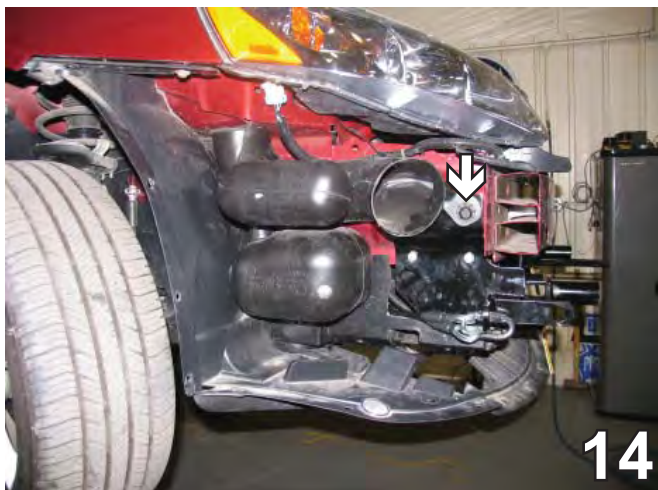
14. Use the existing bolt to reinstall the air baffle and reassemble the push pins.
