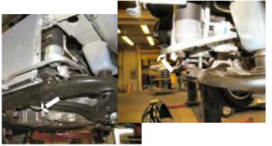
**10.** Lift radiator assembly alignment pin up and out of rubber grommet and push assembly back toward the engine. This will open frame area to allow proper installation of baseplate.
