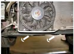
**9.** Using the 10MM socket, remove the two metric bolts from the lower fan assembly, pull fan assembly down to remove from radiator and set aside.
