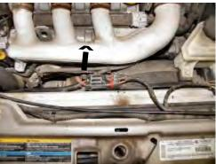
**7.** Pull electrical coupler on top of radiator toward driver's side to release from bracket and unplug.
