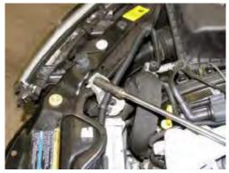
8. Remove the metric bolt from radiator bracket with the 10MM socket and set bracket aside.
