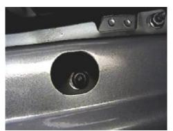
5. Using the 13MM socket, remove six metric bolts from metal bumper, pull forward and set aside. <u>NOTICE:</u> Pull air baffle tube straight down on passenger's side to release and expose inner frame area, set tube aside.
