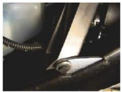
**3.** Remove push pin from fascia support. Using the 10MM socket, remove metric bolt and set aside. Factory fascia support will not be reinstalled.
