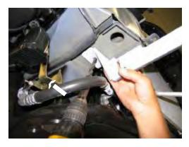
13. Using the baseplate as a template, drill the lower hole into bottom of frame rail, both sides. When drilling holes into the bottom of frame, be aware of coolant line on passenger's side. Insert nut plate into hole on bottom side of frame to align with drilled holes tighten the 3/8-16 hex bolts and lock washers on both side according to drawing on last page. Be sure and use loctite on all bolts before tightening. Torque all bolts according to torque chart in the General Instruction sheet.
