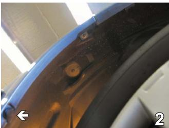
Remove one push pin from the edge of the fascia just forward of the front tire. Do this to both sides, the driver's side is shown. Set push pins aside to be reinstalled later.
