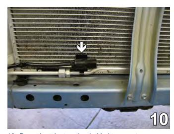
Press the tabs together behind temperature sensor bracket to release sensor and set senor up out of the way to be reinstalled later. When using power drills be aware of the dangers of torque and drill bit length.
