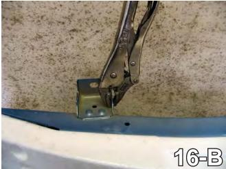
16. Set metal bumper upside down on bench, as shown in 16-A. Cut inside webbing with a reciprocating saw. Do this to both sides of the vehicle. Using he vise grips, bend webbing flat with the bottom of metal bumper see 16-B. Do this to both sides of the vehicle.
