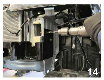
14. Using the baseplate as a template, drill all holes into the frame with the 13/32" drill bit. Do this to both sides of the vehicle.
