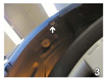
Using a Phillips screwdriver, remove Phillips screw from fascia corner just above front tire in wheel well. Do this to both sides of the vehicle, the driver's side is shown. Set these screws aside to be reinstalled later.
