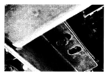
2. Using existing bolts hold baseplate in place and tighten all bolts. Be sure and use loctite on all bolts before tightening.
