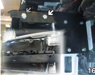
16. Place baseplate between the endplates (see inset). Insert 1/2-13 x 1 1/4" bolts into the endplate's upper holes. Tighten the forward most bolt (see grey arrow) and 1/2" lock washer to the weld nut in the crosstube. Tighten the other upper bolt (see white arrow) to the 1/2" lock washer and 1/2-13 hex nut. Remove the remaining four bolts, apply Loctite, reinsert and tighten. Do this to both sides of the vehicle.
