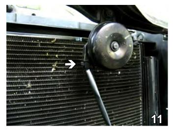
11. Disconnect the electrical connection from the horn by pressing it's tab to release it. Do this to both sides of the vehicle. Set the horn's electrical cables aside to clear the area for baseplate installation and to be reinstalled later.
