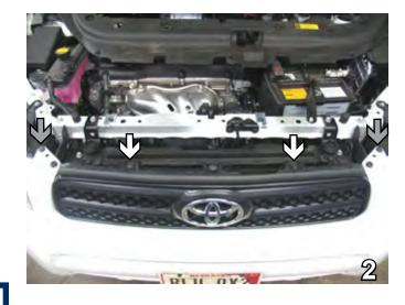
2. Remove two pushpins from the upper corners of fascia (see grey arrows). Above the grille, remove two pushpins from the top of fascia (see white arrows). Set pushpins aside to be reinstalled later.
