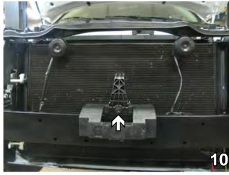
10. Using the 10mm socket, remove one metric bolt from the fascia support molding on top of the metal bumper. Remove fascia support molding and the styrofoam around it. Set both aside to be reinstalled later.
