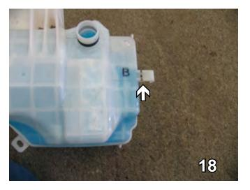
18. Before reinstalling the washer reservoir, using a hack saw blade cut the tab off as shown by the dotted line.
