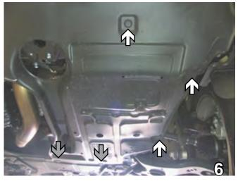
6. Remove five pushpins from the belly pan's driver's side (shown). Remove three pushpins from the passenger's side. Pushpins with grey arrows are found on driver's side only. Pull belly pan down to remove. Pull fascia forward to remove. Set belly pan, fascia and pushpins aside carefully to be reinstalled later.
