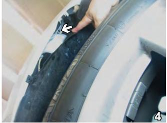
Push wheel well cover aside to expose top edge of fascia. Remove one metric bolt using the 10mm socket. Do this to both sides of the vehicle. Set bolts aside to be reinstalled later.
