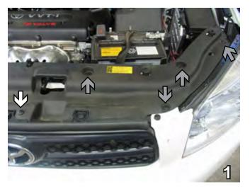
1. Remove four pushpins from the radiator cover (see grey arrows). Do this to both sides of the vehicle. Remove one pushpin near the front and center of radiator cover (see white arrow). Pull up on radiator cover to remove. Set pushpins and radiator cover aside to be reinstalled later.
