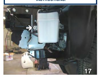
17. Reinstall the air baffle. The brackets are in their original position, but the left side bracket is now over the endplate.
