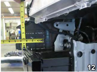
12. On the air dam, mark a 3" vertical line that is 4 1/4" inches from the front of the air dam. Mark two horizontal lines that reach the front of air dam. The lower line runs above the bottom rib (flush with the bumper). Using the hack saw, cut the marked area. Note: Do not remove the bottom or side rib - cut above or to the inside of the rib. Do this to both sides of the vehicle.
