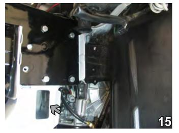
15. Insert 3/8" lock washers and 3/8-16 hex nuts through frame rail opening (see grey arrow) and align to drilled holes. Insert 3/8-16 x 1" bolts and hand tighten (don't use Loctite yet). Do this to both sides of the vehicle.
