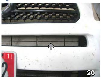
20. With the fascia on a hard, flat surface, use the hack saw blade to remove the second rib in from the outside edge of the grille style.
