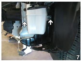
On the driver's side, use the 10mm socket to remove two metric bolts from the air baffle brackets. Remove air baffle. Set bolts and air baffle aside to be reinstalled later.
