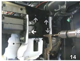
14. Align bottom of the endplate flush with the bottom of the frame and with the pre-existing hole of the frame (see white arrow). The endplate's angled top edge points to radiator. Clamp with vise grips. With the endplate as a template, drill four holes into frame (see grey arrows) using the 13/32" Carbide drill bit. Do this to both sides of the vehicle.
