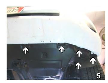
Along the bottom edge of fascia, remove five pushpins (three in the center and two from each tire guard) using the 10mm socket. Do this to both sides of the vehicle. Set pushpins aside to be reinstalled later.
