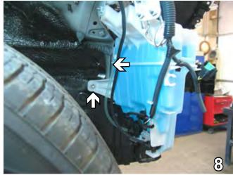
8. On the passenger's side, disconnect electrical connections from the side of washer reservoir and plug the reservoir. Push wheel well cover aside to remove one metric bolt behind the reservoir (see upper white arrow) using the 10mm socket. Remove one metric bolt from the side reservoir bracket (lower white arrow) using the 10mm socket. Set bolts aside to be reinstalled later. If applicable, disconnect fog lights.
