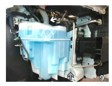
Disconnect the tube from the top of washer reservoir (see white arrow). Using the 10mm socket, remove one metric bolt from the lower bracket of reservoir. Remove washer reservoir. Set bolts and reservoir aside to be reinstalled later.
