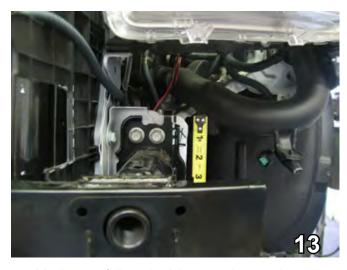
13. Mark a 1 1/2" vertical line starting on the front of the frame rail, flush with the side of the frame rail, moving down over the bumper bracket. Then, mark horizontally from the bottom of the vertical line to the outside of frame rail. Using the reciprocating saw, cut the marked area.
