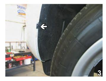
On outside edge of wheel well, turn screw 90 degrees with the flat screwdriver to remove.
