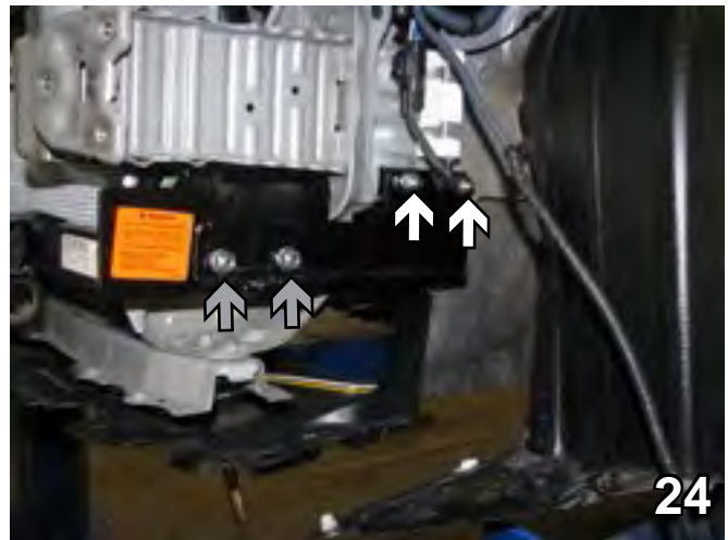
24. Loosen the front two bolts (gray arrows). Insert in the back 3/8"-16 x 1 1/2" bolts, the spacer plates, 3/8" lock washers and 3/8" hex nuts. Loctite Red all bolts and tighten. Then install 3/8" lock washers onto the front two (2) 3/8"-16 x 1" bolts (gray arrows) and 3/8" hex nuts, Loctite Red all bolts and tighten. Do this on both sides.
