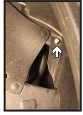
Loosen the wheel well liner by removing the lower screw with a 10MM socket (left) and removing the push pin in the wheel well (right). Pull back the liner to access the frame. Do this on both sides of the vehicle.
