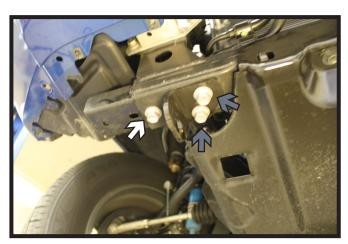
Using a 17MM socket, remove the bolts from the frame extensions. There is one (1) on each side (white). Set the extensions aside they will not be reinstalled.
