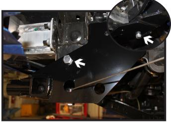
10. Install the spacer tube thru the frame on the driver side. Position the DS baseplate onto the frame and install the 1/2" x 4" bolt and hardware. Do not fully tighten. Install the 1/2" hardware into the bottom existing hole (inset) and fully tighten the bolt.
