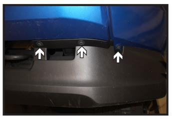
1. Using a 10MM socket, remove the four (4) screws from the inside edge of the lower valance. There are two (2) on each side (left). Continue along the outside of the valance removing the nine (9) screws along the edge (right). Set the valance aside.
