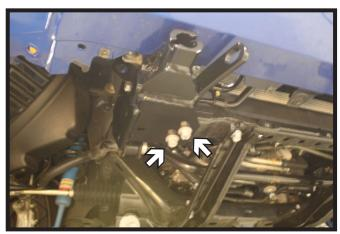
7. Position the PS baseplate onto the vehicle and install the two (2) existing tow hook plate bolts thru the baseplate into the frame. Do not fully tighten.
