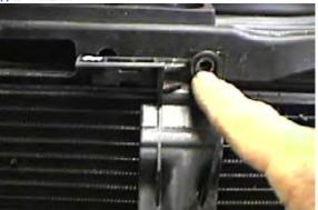
**7.** Using the T-30 Torx, remove the five torx bolts from fascia support.
