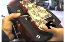
Note: If using the Bx8869,remove electronic circuit board off the back of light assembly, photo to the left shows socket location.
