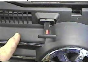
1. Remove the hood release handle by lifting retainer clip pull forked end apart, pull forward, and set aside.
