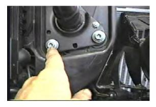
**9.** There are three torx bolts to remove from bumper mounts with the T-45 Torx, each side.
