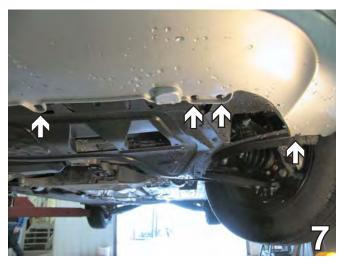
Use the 25 Torx socket, remove the four metric bolts from the lower edge of the fascia. Do this on both sides of the vehicle. Set bolts aside to be reinstalled later.
