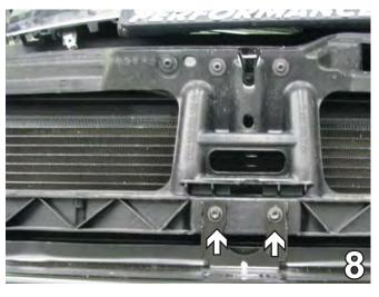
Remove the two Torx bolts just above the middle of the metal bumper with the 30 Torx socket.
