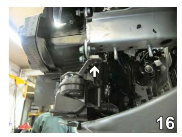
16. Using the 12MM socket, remove the metric bolt from the horn bracket. Unplug the electrical connections, set the horn and bracket aside. Do this on both sides of the vehicle.
