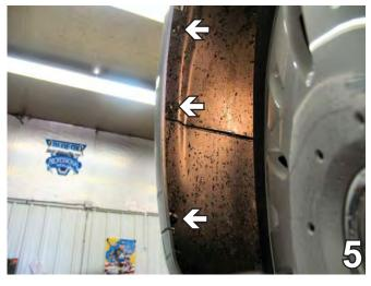
Remove three metric bolts just forward of the front tire on the edge of the wheel well, using the 25 Torx socket. Do this on both sides of the vehicle. Set bolts aside to be reinstalled later.
