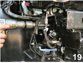
19. Using the baseplate as a template, drill the holes in the side of the frame rail with the 13/32" drill bit. Do this on both sides of the vehicle.
