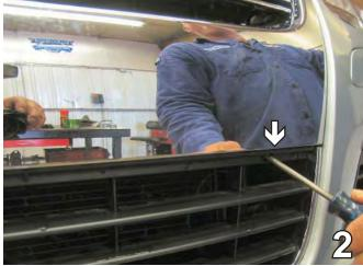
2. Remove the two phillips screws from the lower grille, one on each side. Set screws aside to be reinstalled later.
