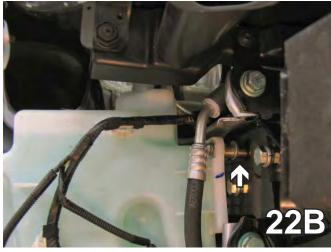
22. Put the washer reservoir in place on the back two studs (22A) and install the two hex nuts (Do not tighten). Replace the front metric bolt with the 6MM hex bolt provided. Install spacer tube, flat washers and lock washer provided (22B). Be sure that the webbing does not touch on the back side of the reservoir. This will prevent webbing from rubbing a hole in the reservoir tank (22A). Reconnect all the electrical and fluid lines to the reservoir (22B).
