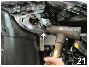
21. Using the hammer, tap the webbing toward the back of the vehicle 3/8", just behind the washer reservoir, on the passenger's side. This will prepare the area for reinstallation of the washer reservoir.
