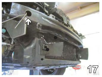
17. Using the 1 1/4" hole saw, cut a hole on the front of the metal bumper just forward of the center of the frame end. Do this on both sides of the vehicle. This will allow access to the inside of the frame end to insert the nut plates for the base plate installation.
