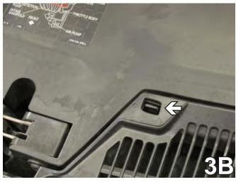
3. Using the flat screw driver, pry up the front edge of the grille, just inside the headlight assembly, to release the corner (3A). Pull the two clips forward to release the upper grille portion while pulling the upper grille forward and set aside to be reinstalled later (3B driver's side clip).
