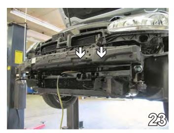
23. Reinstall both horns and their brackets. Reinstall the styrofoam on the front of the metal bumper.
