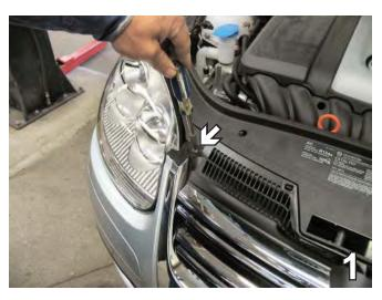
Using the 25 Torx socket, remove the metric bolt just inside of the headlight assemblies. Do this on both sides of the vehicle. Set bolts aside to be reinstalled later.
