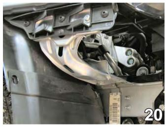
20. Insert the nut plate into the drilled hole on the front of the bumper to align with the drilled holes in the frame. Tighten the 3/8" bolts and lock washers on both sides. Keep the base plate attachment tabs level with the vehicle. Be sure to use Loctite red on all the bolts before tightening. Tighten all the bolts according to Torque Chart in the General Instruction Sheet.
