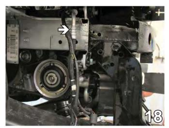
18. Slide the base plate onto the side of the frame with the attachment tabs down. Push the base plate back toward the rear of the vehicle while lifting the cross tube up. The bottom edge of the end plate should be even with the bottom edge of the frame. Align the top center hole with the existing bolt location for the front of the washer reservoir on the passenger's side, clamp to the frame with vise grips.
