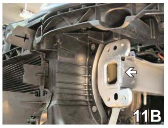
11. Measure from the top edge of the frame end down and mark 2" and 5 1/2" on the side of the frame webbing. Using the reciprocating saw, cut the webbing to the side of the frame rail and make a vertical cut flush with the side of the frame between the first two cuts. Remove this area on both sides of the vehicle to prepare for the base plate installation. Using a good quality spray paint, coat the cut edges to prevent corrosion. Do this on both sides of the vehicle.
