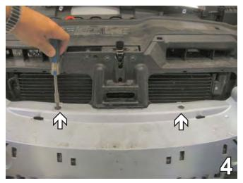
4. Below the grille, on the top of the metal bumper, are two Torx bolts to remove with the 30 Torx socket. Set bolts aside to be reinstalled later.
