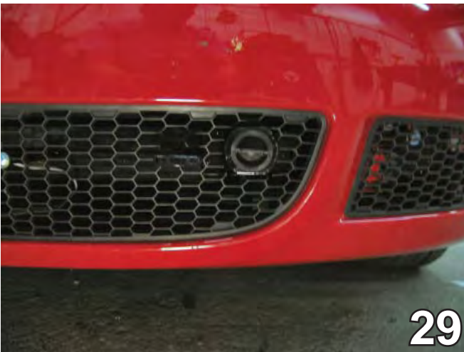
29. Reinstall the fascia and center grille, inserting all screws, pushpins, and bolts. Align the fascia to its original position and, using a diagonal cutter, trim necessary openings in the grille for attachment tabs, convenience links, and electrical rods. The installation of the baseplate is complete.
