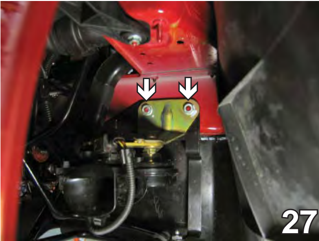
27. Reinstall horn bracket and metal bumper.
