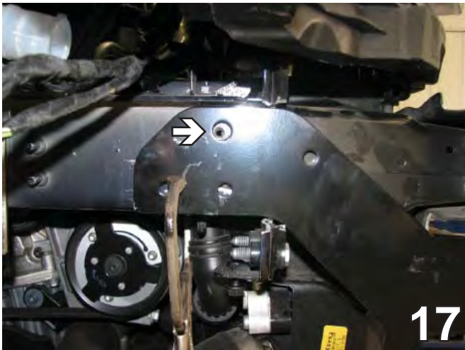
17. Slide the base plate onto the side of the frame with the attachment tabs down. Push the base plate back toward the rear of the vehicle while lifting the cross tube up. The bottom edge of the end plate should be even with the bottom edge of the frame. Align the top center hole with the existing bolt location for the front of the washer reservoir on the passenger's side, clamp to the frame with vise grips.
