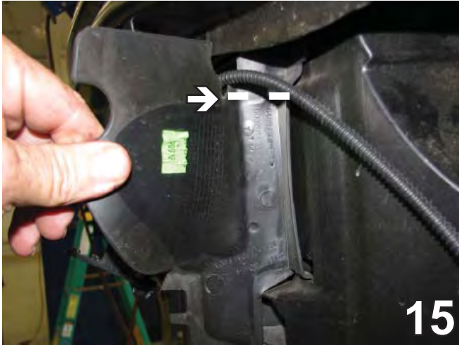
15. Move the hose and mark the air dam just below the metal bumper. Using a utility knife, cut and remove that portion. Do this on both sides of the vehicle.
