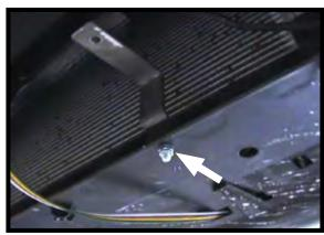
14. You may place the breakaway bracket anywhere on the vehicle frame. Using a 9/32" drill bit, drill a hole into the frame.
