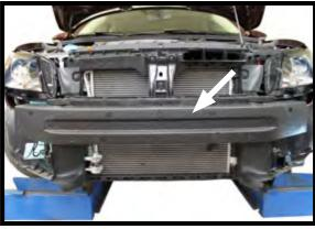
Pull the styrofoam bumper padding off and place to the side for reinstallation after the baseplate is installed.
