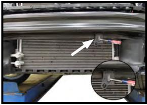
7. On the driver side, lift the tab up using a flat screwdriver and slide the temperature sensor off. Set aside for reinstallation later.
