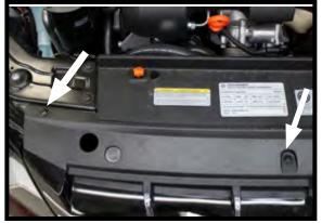
1. Using a Torx 25 remove the three (3) screws that are located in the front area, underneath the hood. There is one (1) screw located on the outer edge of the driver side and two (2) on the passenger side. On the passenger side, one (1) is located on the outer edge and the other is located just to the left of the center of the vehicle.
