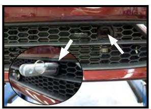
13. Hold the front fascia as close to the original state as possible and mark where the cutout for the convenience links, attachment tabs and breakaway switch, is so equipped, will be located.
