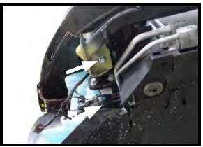
10. Verify the baseplate is level and install the 3/8"-16 x 1-1/4" hex head bolts, 3/8" lock washers and 3/8" flats washers on the bottom slot. Do this on **BOTH** sides of the vehicle.
