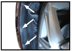
Remove the three (3) screws in the front wheel well area using a Torx 25.
