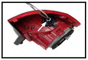
Drill a 1" hole to install the 3 wire automotive socket.
