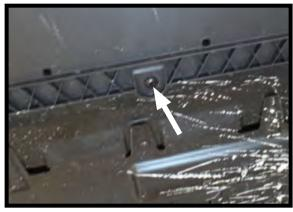
4. On the underside of the front fascia there are seven (7) screws that need to be removed using a Torx 25. There are three (3) on both the driver side and the passenger side, plus one (1) in the center of the vehicle.
