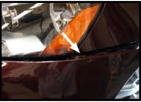
5. Gently, yet firmly, pull outward on the front fascia to remove. Next, remove headlights on **BOTH** sides of the vehicle.
