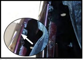
Pull the wheel well liner back. Using a Torx 25 remove the screw that is located underneath. Do this on **BOTH** sides of the vehicle.
