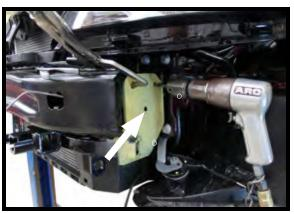
11. Using a 13/32" drill bit and using the baseplate as a template, drill the three (3) sides holes. Do this on **BOTH** sides of the vehicle.
