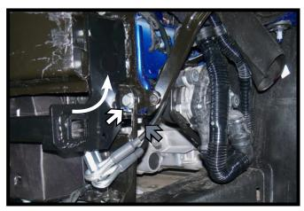
14. Slide the notched braces onto the baseplate and rotate into position on the vehicle. Start the outer existing brace bolt (white) and a 8MM-1.25 x 30MM bolt with a 8MM flat and lock washer into the underside hole of the baseplate (gray). Do this on both sides of the vehicle. Level and clamp the baseplate into position.
