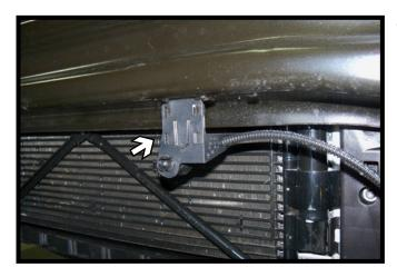
8. Remove the air temperature sensor from the bumper and set aside.
