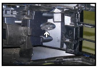
20. On the backside of the fascia, trim off material from the rib for baseplate clearance. Do this on both sides of the fascia.
