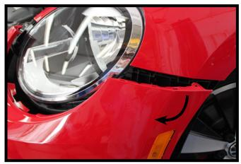
When removing front fascia, pull straight out and unhook both the side marker and running light wiring on both sides of vehicle.
