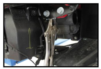
11. Remove the tab the horn was attached to flush with the body, either by bending back and forth with vise-grips as shown or using a reciprocating saw. Repeat on other side of vehicle.
