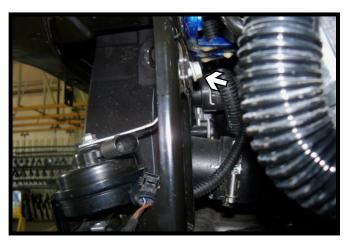
Using a T50 Torx, remove the screw from the backside of the horn bracket.
