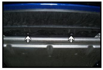
5. Using a T25 Torx, remove the eight (8) screws from the underside of the fascia. There are three (3) on each side and two (2) in the middle.
