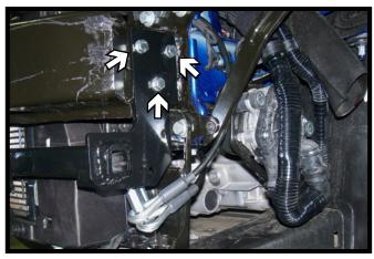
15. Using a 13/32" drill bit, drill the three (3) holes thru the frame. Install 3/8"-16 x 1-1/4" bolts with lock washers into the holes and 3/8"-16 nut plates on the inside of the frame. Do this on both sides of the vehicle. Fully tighten all fasteners.
