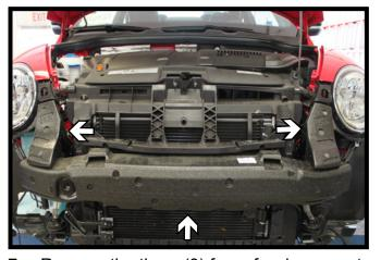
Remove the three (3) foam fascia support pieces. DO NOT discard, these will be reinstalled later.
