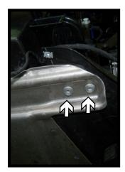
10. Using a 16MM socket, remove the two (2) bolts from the upper section of the brace (left). Using a T50 Torx, remove the two (2) screws from the underside of the brace (right). Do this on both sides of the vehicle.
