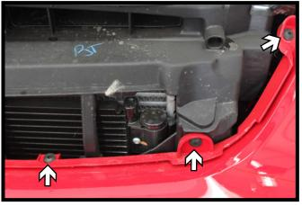
2. Using a 25 Torx, remove the six (6) screws at the top of the fascia. There are three (3) on each side.
