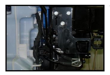
17. Attach the permanent baseplate safety cables to the provided convenience link on the baseplate. The photo shows the recommended installation of the cables to frame of vehicle. Additional options may interfere with suggested mounting; in this case, secure the cables to a solid piece of the frame as described in the instructions included with the permanent baseplate safety cables. Be sure the safety cables do not rub against any hoses or moving parts. Do this on **BOTH** sides of the vehicle.
