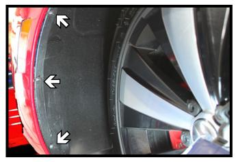
3. In the wheel well, use a T25 Torx to remove the three (3) screws. Do this to both sides of the vehicle.
