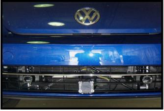
21. Hold the fascia as close to its original position, mark and trim the fascia around the convenience links and attachment tabs. Reinstall the fascia and fascia cover.
