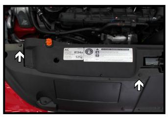
Remove the four (4) push pins from the top edge of the radiator cover. There are two (2) on each side. Then remove cover from vehicle.
