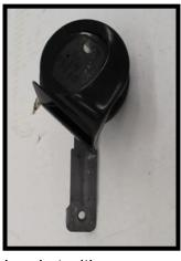
18. Flatten out the horn bracket with a hammer on a solid surface. Then remove the side tab with pliers or vise-grips by twisting back & forth (shown above to left). Bracket should look like right hand picture when done. Repeat on other horn.
