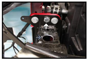
12. Install a 1/2"-13 x 1-1/2" bolt and 1/2"-13 whiz lock nut in the existing frame hole (white).
