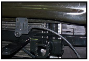
16. Reinstall the air temperature sensor.
