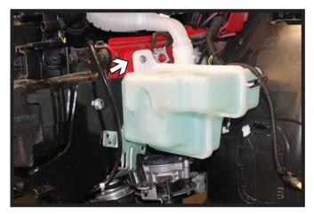
17. Reinstall the washer reservoir using four (4) flat washer on the top left stud in between the tank and frame. This will space the tank out so it clears the baseplate.
