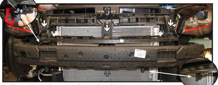
Remove the styrofoam support from the face of the bumper (gray).
