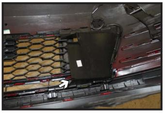
19. On the backside of the fascia, remove the plastic covers on both sides.
