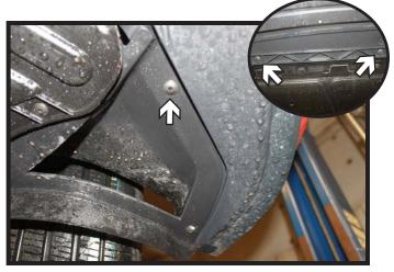
Using a T25 Torx, remove the seven (7) screws from the underside of the fascia. There are two (2) on each side in each corner and three (3) across the middle.
