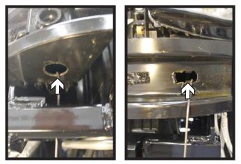
13. Using a 1-1/4" hole saw, drill an access hole on the underside of the bumper on the passenger side only (left).
