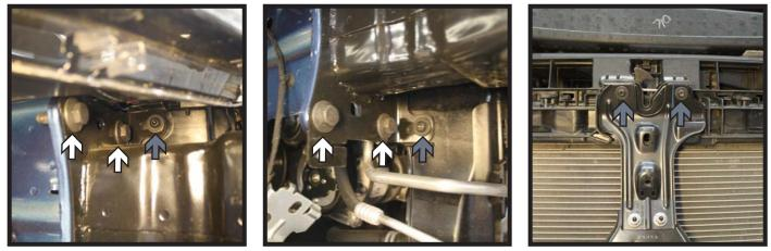
6. Using a 16MM socket, remove the eight (8) bolts from the bumper. There are four (4) on each side, two (2) on top & two (2) on bottom (white).
