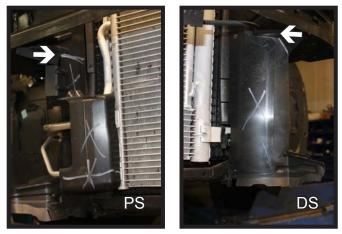
12. Trim the plastic shielding off just below the bumper on both sides of the vehicle. The shielding is not reinstalled.
