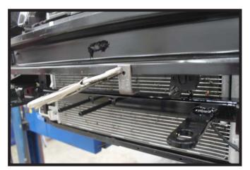
Optional Breakaway: Position the bracket in the desired location along the bottom lip of the bumper. Clamp and drill a 5/16" hole thru the bumper. Install the bracket to the vehicle with the supplied 1/4" hardware.
