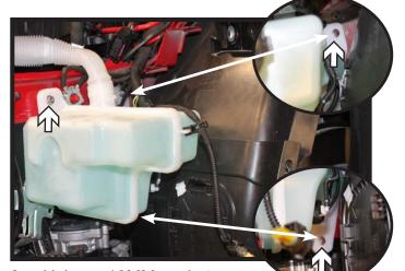
8. Using a 10MM socket, remove the three (3) nuts from the washer reservoir. Disconnect/plug all lines and set the reservoir aside.
