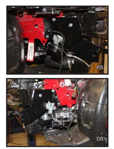
15. Prior to drilling and installing the remainder of the baseplate bolts, flatten the three (3) tabs of the horn brackets (upper left) so it will sit flat on the face of the side plate. Also it may be necessary to ream out the slot to accommodate the hardware (lower left).
