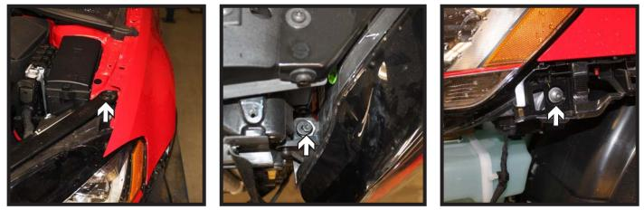
Using a T30 Torx, remove the three (3) screws from the driver side headlight. There are two (2) on the top side (left & middle) and one (1) on the side (right).
