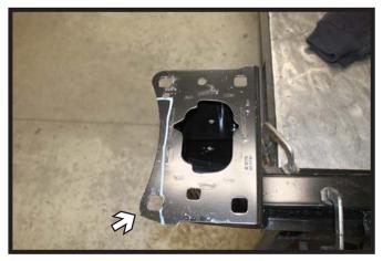
10. Temporarily reinstall the bumper. Mark the backside of the mounting flange along the cuts of the frame. Remove and trim these areas on both sides of the bumper with a reciprocating saw.
