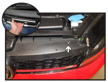
Using a T25 Torx, remove the two (2) screws from the top edge of the grille. There is one (1) on each side. Unsnap the grille from the vehicle and set aside.
