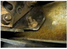
**2.** Remove two metric nuts from inner bumper bracket with the 19MM socket, both sides.
