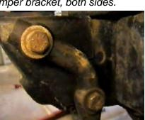
3. Remove two metric bolts from tow hook with the 19MM socket and wrench, both sides. Tow hooks will not be reinstalled.
