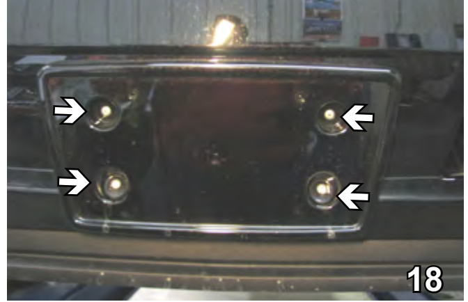
18. Cadillac Escalade: On the front of the car after the baseplate is installed, drill out the pop rivets on the license plate bracket with a 3/16" drill bit and replace them with plastic pop rivets.
