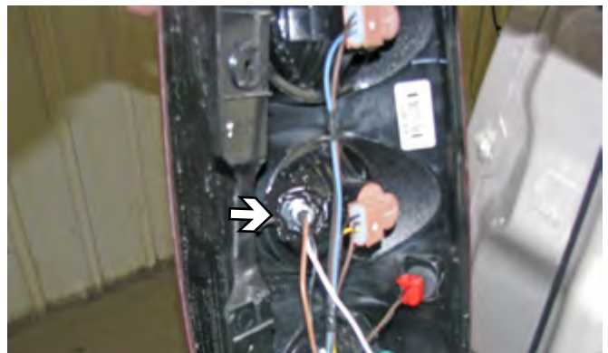
GMC Yukon- Possible location for the Bulb and Socket Wiring Kit (BX8869).
