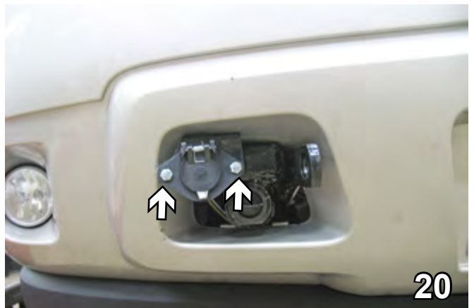
20. All Others: The photo to the left shows the recommended location of the electrical connector.
