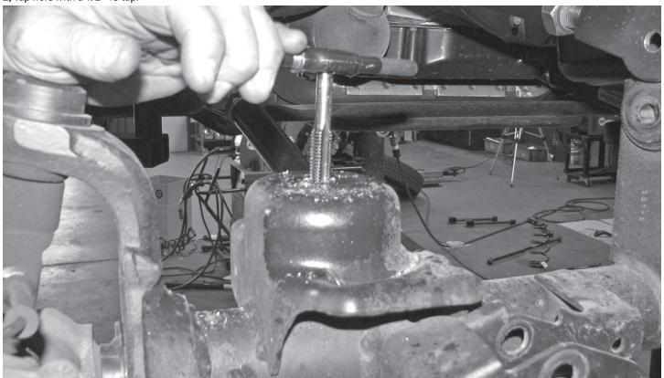
**3.** When installing springs, insert the bump stop and spacer inside the spring prior to installation. Install spring then insert bolt and washers through spring and bolt bump stop kit down (use red loc-tite).
