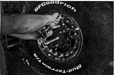
Step 8: Place provided nuts onto the stud extenders and tighten down to 45ft lbs.
