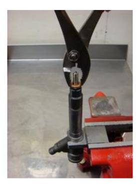
5. Using a 15mm wrench, remove the nozzle nut. Once you have removed the nozzle nut you can remove the nozzle, but BE CAREFUL not to lose the small puck which can sometimes stick to the nozzle. The puck fits into the small recess right in the middle of the injector body and lays flat.
