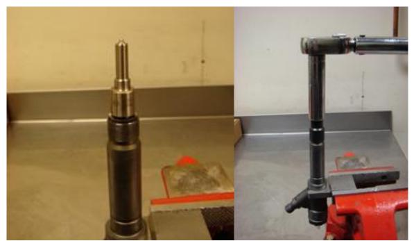
9. Use supplied grease packet to hold the new copper washers onto the injector. Don't be afraid to use it liberally to make sure the washer does not fall off when you are reinstalling the injector into the head.
