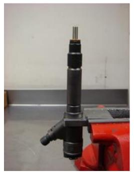
4. Using pliers, remove the copper sealing washer. If you are missing the copper washer be sure to dig it out of the cylinder head before putting the injectors back in. Some carbon buildup may be present and this is normal. Sometimes the carbon may seem excessive but there is no reason to worry. Do not clean the nozzles for us. We use an ultrasonic machine to gently clean the nozzles without damaging them.
