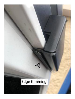
14. Insert bolt and washer from top down of upper mounting plate and thread into outer rail mount. Lower edge with trim should be grabbing underside of hardtop drip rail.
