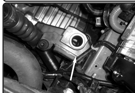
11. Locate the resonator box hole, make sure the OEM grommet is installed and seated properly.
