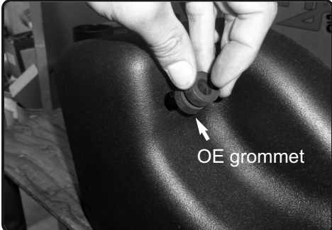
9. Install the OEM grommet to the hole on the air box.
