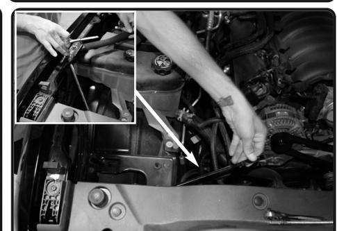
**19.** Loosen the support bar using 10mm socket or wrench. Push back for installation of air box.
