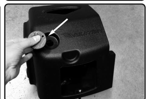
12. Push the Filter Monitor Plug into the Filter Monitor pod on the Injen air box if you are not using the Filter Monitor Kit P/N AC1000
