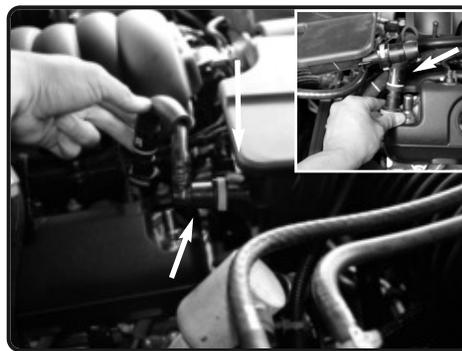
7. Disconnect both of the crank case lines from the air box and engine and remove the hard lines from vehicle.
