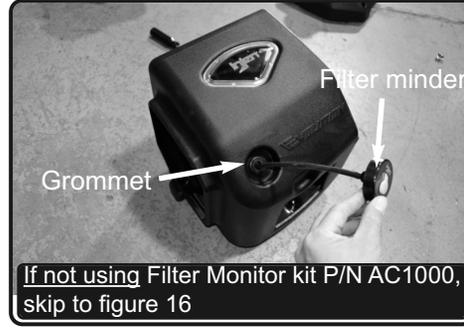
**14.** Install the provided grommet to the hole on air box, now attach the 3mm vacuum line to the filter minder and install the filter minder to the air box. Place hose through the grommet.
