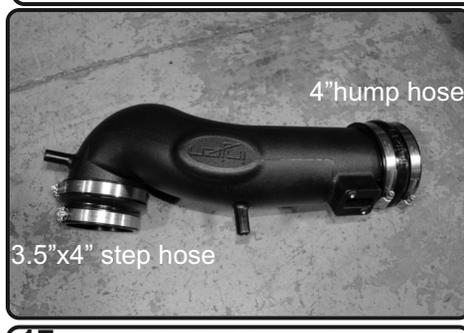
**17.** Install the 3.5"x4" step hose with clamps to the intake tube. Install the 4" hump hose to the intake tube with clamps. *For 6.2L only, use provided 4" straight hose on throttle body.*
