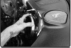
**17.** Once the filter is seated, turn the the filter in either direction a 1/4" turn.
