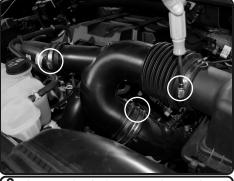
**3.** Loosen the 3 clamps on the stock intake tube using 7mm nut driver.
