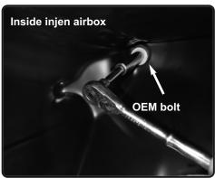
**14.** Use the OE air box bolt to secure the lower Injen air box to the chassis and tighten.
