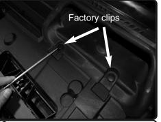
**2.** Remove the two plastic retaining rivets from the air scoop and save for later install.
