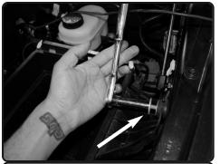
**5.** Loosen the bolt holding in the bottom of the airbox using 13mm socket or wrench. Save bolt for later install.
