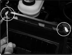
**6.** Pull back the harness from the air box. Pull back vacuum solenoid.
