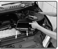
**13.** Install injen air box into vehicle and position to the OEM stand off grommets and to chassi.
