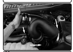
**20.** Install the intake tube assembly into the vehicle and position. Positon the intake tube into the filter and intake pipes.
