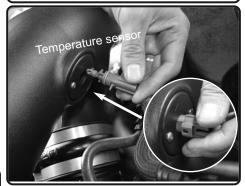
**22.** Install the temperature sensor into the adaptor. Once seated correctly turn and lock into position.
