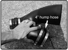
**10.** Install the 4" hump hose to the other end of the intake tube with clamps lprovided.
