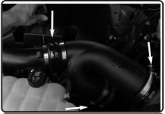
**21.** Adjust for fit, and tighten all the clamps using 8mm nut driver.
