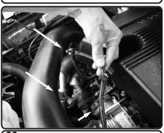
**23.** For the 3.5.L and Raptor models, pull back the Temp harness clips from the in-take tube, this will allow for more length to the sensor. Re-connect Temp harness.
