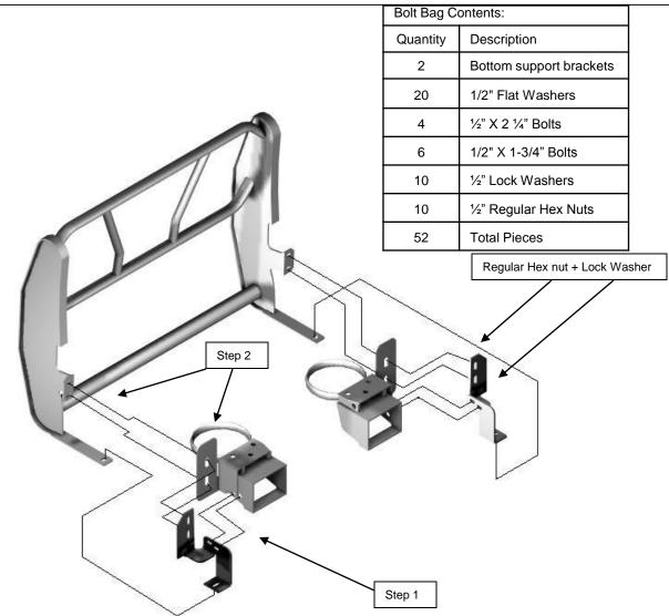
**Step 1:** Install bottom support bracket behind frame horn. NOTE: You must use regular  $\frac{1}{2}$ " hex nuts and  $\frac{1}{2}$ " lock washers on the bolts going through the truck frame!! You will access the bolt head through a small hole located on the inside/bottom of truck frame when you are tightening.
