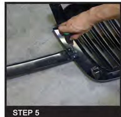
For use with OEM lights - Attach side pieces onto grille using provided hardware (3 phillips head screws per side)
