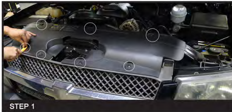
Remove (7) radiator cover fasteners - save for reuse
