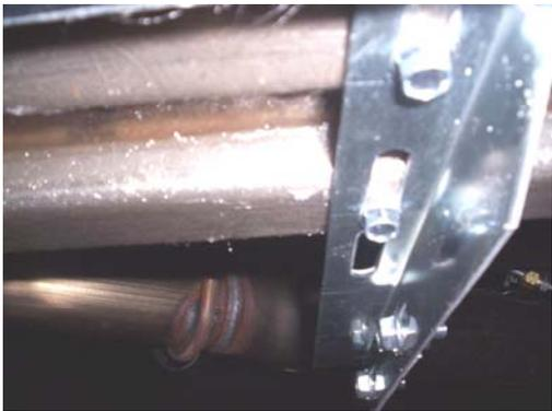
Place the board on the brackets. Using a small jack to hold the board, position it up against the vehicle to achieve the best fit. Slide the channel brackets up to the bottom of the board and attach with self drilling screws. Tighten the bolts holding the channels..
