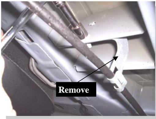
On the driver side at 25" (23" on passenger side) back from wheel well, remove factory bracket holding the emergency brake cable.
