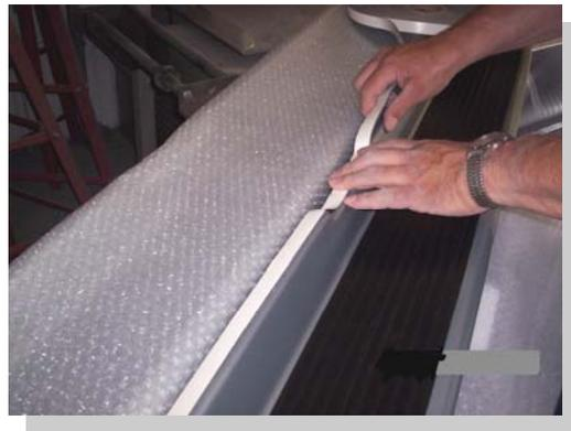
Attach foam tape to the top lip of the board where it meets up with the body. Attach step tread and logo also.
