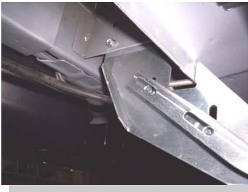
Attach one channel bracket with 5/16 bolts and nuts on each flat bracket. Snug but do not tighten.
