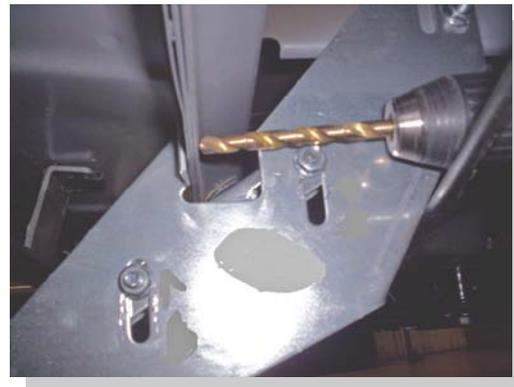
Attach an FL125 with supplied 5/16 bolt and nut through hole where cable bracket was removed. Drill a 5/16" hole from the back side of the pinch weld to line up with the hole in the bracket and attach with 5/16" bolt and nut.
