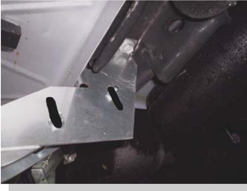
Attach FL127D using bolts removed in step3. From back side of pinch weld drill 5/16" hole through pinch weld to line up with the hole in the bracket. Insert a 5/16" bolt and fasten with nut. Tighten all bolts.
