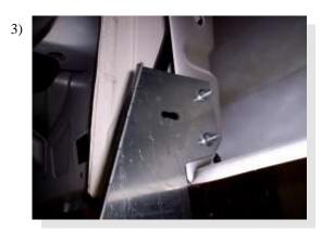
Attach the FL152 bracket to the sidewall support using 5/16" bolts and nuts.
