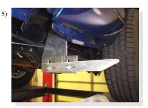
Attach a 3124F angle bracket to the FL152 with 5/16" bolts and nuts. Snug but do not tighten at this time.
