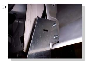
Attach the FL152 bracket to the box sidewall support using 5/16" bolts and nuts.
