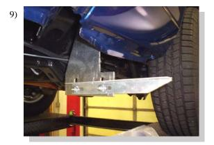
Attach one 3124F (short angle) to the front bracket and one 3124J (long angle) to the rear bracket with 5/16" bolts and nuts. Snug but do not tighten. (Short box shown)
