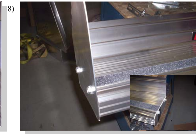
Attach stone guard and end cap to running board using 3/8" self threading bolts.
