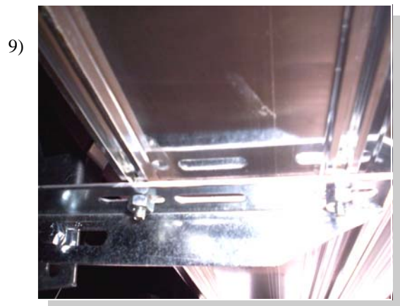
Place the board on the brackets with the bolts through the slots. Fasten with 1/4" nuts. Note: riser of box board tucks behind bedside in order to line up with 2" riser of cab board.
