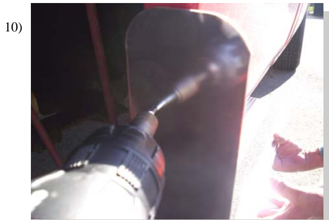
Make sure board is lined up with cab board. Use one self drilling screw to attach the stone guard to the fender lip. Make sure the board is level, then use remaining 2 screws to finish attaching stone guard to fender lip.
