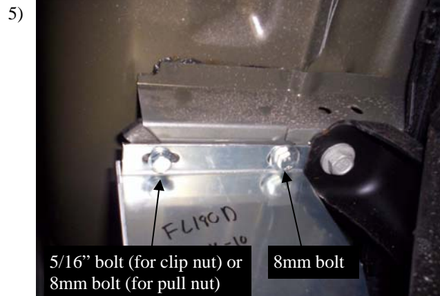
Install FL180D & P using 5/16" flanged bolt (for clip nut only) and 8mm bolt and washers, as in Fig. 5.
