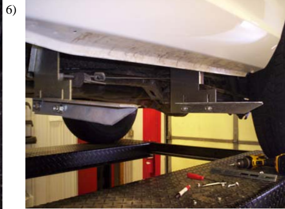
Attach a 3124F angle bracket to the FL181 and FL180D & P with 5/16" bolts and nuts. Snug but do not tighten at this time.
