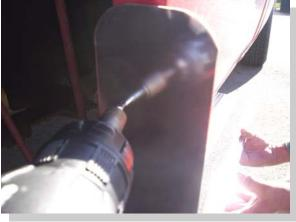
Make sure board is lined up with cab board. Use one self drilling screw to attach the stone guard to the fender lip. Make sure the board is level then use remaining 2 screws to finish attaching stone guard to fender lip.
