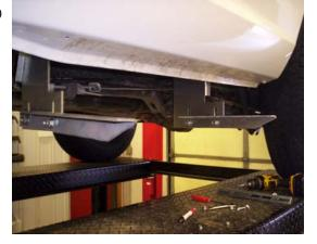
Attach a 3124F angle bracket to the FL181 bracket with 5/16" bolts and nuts. Snug but do not tighten at this time. **Picture shows** long bed with extra bracket not needed in short bed.
