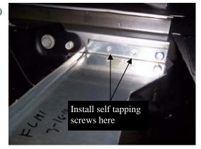
Attach the FL181 bracket to the front bed cross member support, using 5/16" bolt, as shown in **Fig. 2.** Next install self tapping screws into the other holes in the bracket to the cross member.
