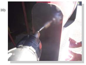
Use one self drilling screw to attach the stone guard to the fender lip. Make sure the board is level. Use remaining 2 screws to finish attaching stone guard to fender lip. Tighten any and all loose bolts. Repeat all steps for opposite side.
