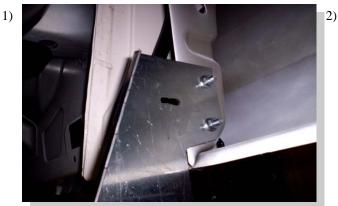
Attach the FL185 bracket to the front bed sidewall support, using the factory bed support bolts. Remove them then reinstall.
