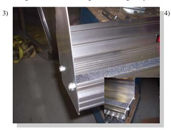
Attach stone guard and end cap to running board using 3/8"self threading bolts.
