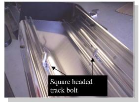
Insert one square headed track bolt into both tracks for each bracket.
