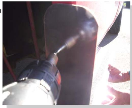
Use one self drilling screw to attach the stone guard to the fender lip. Make sure the board is level. Use remaining 2 screws to finish attaching stone guard to fender lip. Tighten any and all loose bolts. Repeat all steps for opposite side.
