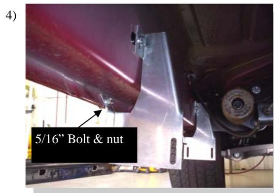
Attach brackets to vehicle by inserting the retaining nut in the factory ob-round hole and using one 5/16" bolt and nut through the pinch weld.
