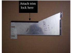
Cut trim lock to 12" and attach to FL206D and P as shown in Fig 3.
