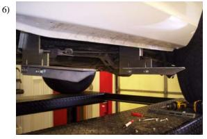
Attach a 3124F angle bracket to the FL185, and attach 3124G (the longer one) to FL206D/P with 5/16" bolts and nuts. Snug but do not tighten at this time.
