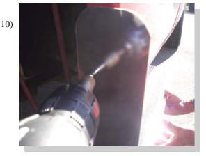
Use one self drilling screw to attach the stone guard to the fender lip. Make sure the board is level. Use remaining 2 screws to finish attaching stone guard to fender lip. Tighten any and all loose bolts. Repeat all steps for opposite side.
