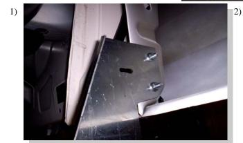
Attach the FL185 bracket to the front bed sidewall support, using the factory bed support bolts. Remove them then reinstall.
