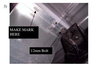
In front of rear wheel, above front leaf spring shackle on the bed cross member, attach FL206D/P with 12mm flanged bolt. Just snug bolt. Make a mark in the center of the slot so you can turn bracket and drill a 1/2" hole.
