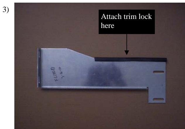
Cut trim lock to 9-3/4" and attach to FL222D & P as shown in Fig 3 .
