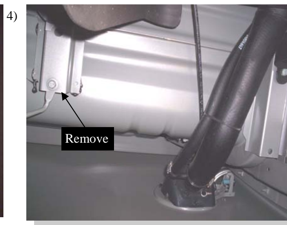
In front of rear wheel, above front leaf spring shackle, on the bed cross member, remove factory bolt holding fender brace. Save bolt you will need it later.
