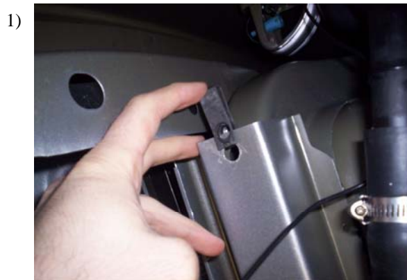
Locate the front bed cross member and install clip nut as shown in Fig. 1 .
