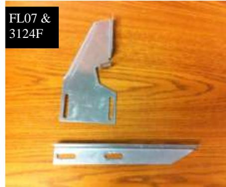
**STEP 2:** Assemble FL07 and 3124F w/ 5/16" nut and bolt as shown. Hand tight to allow for running board adjustment once running board is on
